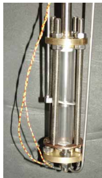
Fig. 2 A high-pressure cell for the growth of solid He.
